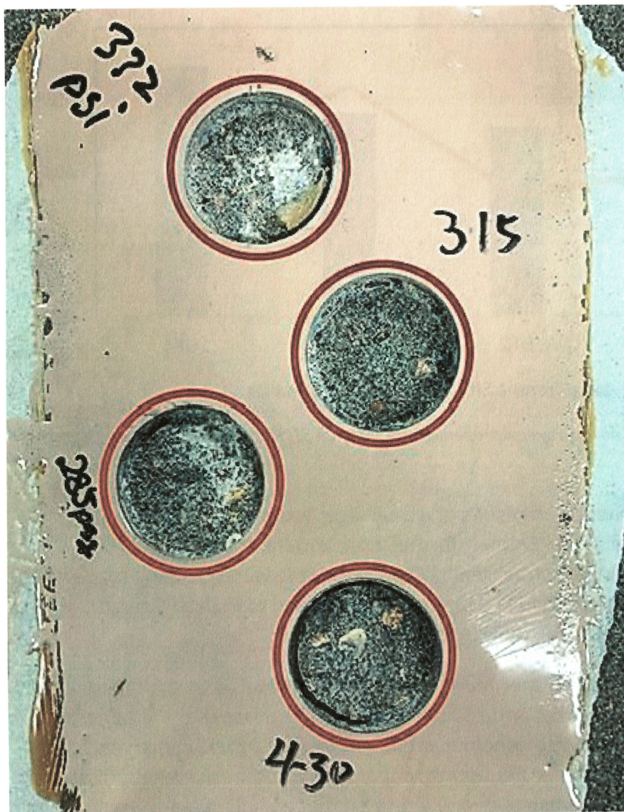
Figure 2. 2K STPE/epoxy adhesion strength testing results. Red circles indicat... »
